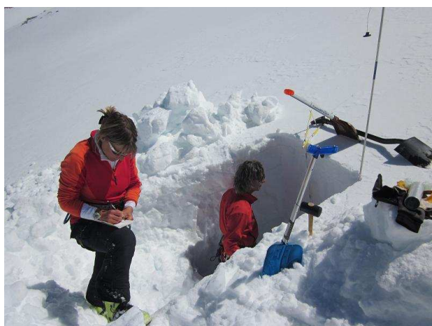
Figures 1/2. On the left snow pit for the stratigraphic and density profile analyses of winter accumulation (picture Hartmann Stuefer, May 5. 2010) and right ice hole in the frontal part of the orographic right tongue (picture Roberto Dinale, August 25. 2010) of the Westlicher Rieserferner/Vedretta occidentale di Ries glacier (I4L00123312).
