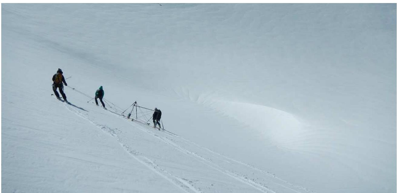
**Figure 1.** Matscher Ferner / Vedretta di Mazia: Ice thickness measurements at June 12, 2013 (IGF Institute of the Austrian Sciences Academy).
